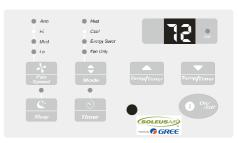
Note: Tap or hold either  $up(^{\land})$  or down(v) button until the desired temperature is seen on display. This temperature will be automatically maintained anywhere between 61F (16°C) and 86F (30°C) for both cooling and heating modes. If you want the display to read the actual room temperature, select the Fan Only mode.
